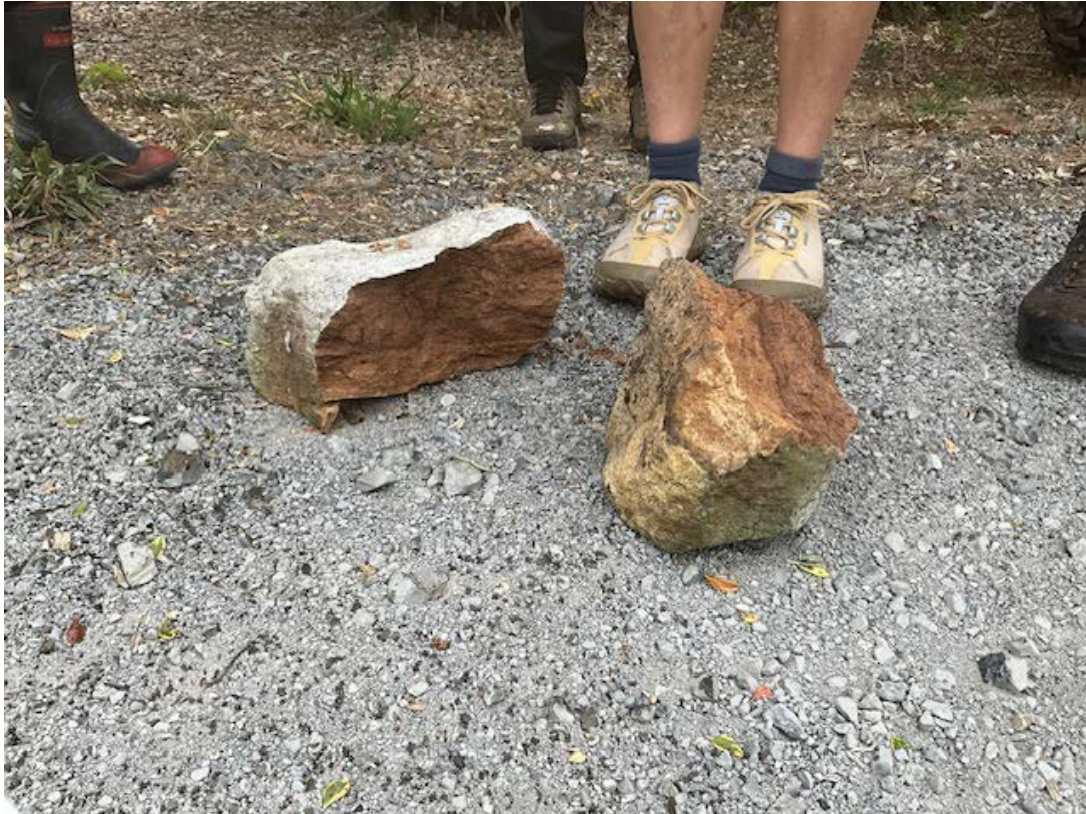
Figure 11: Example of silica pan extracted from ridgeline podzol soils at the example location.
