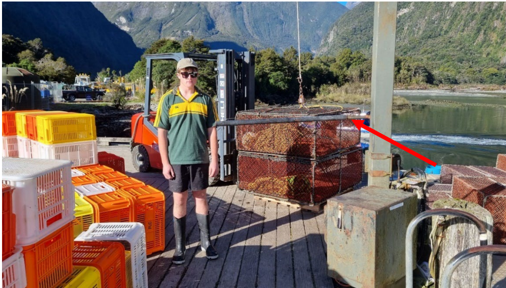
Figure 5: Example of crane horizontal bar hazard (red arrow) and cranes lifting cages weighing approximately 100kg each which can cause crushing injuries.
