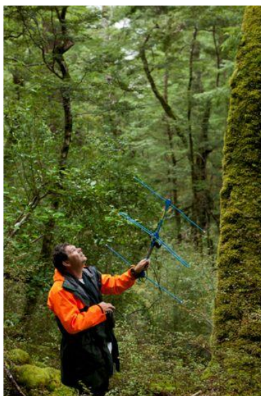
Figure 75. Tracking a bat with a 3-element yagi antennae (photo: S. Bernert).
