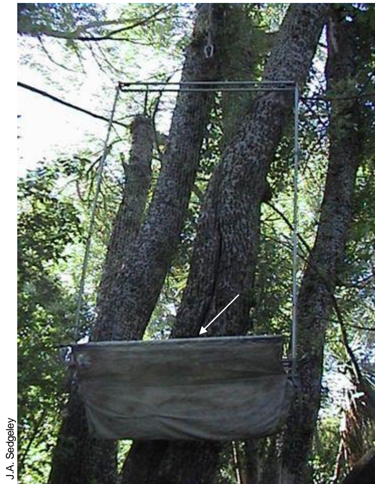
Figure 38. Harp trap placed outside long-tailed bat roost. Arrow indicates the bottom of the roost entrance.
