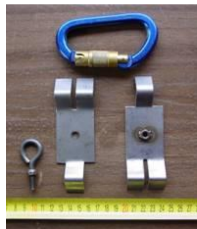
Figure 31. Attaching bridle to suspend harp trap. Illustration from harp trap instruction manual.
