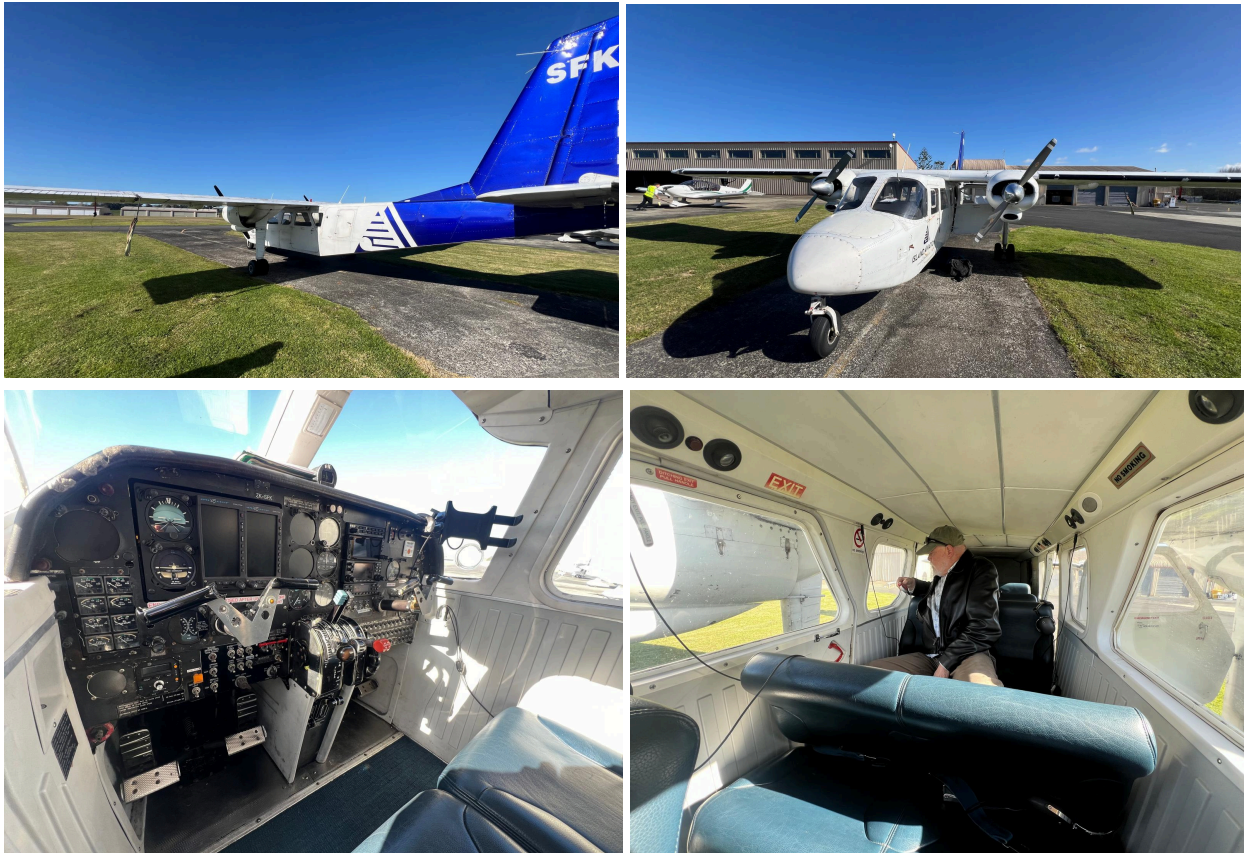
Image Set 2: Britten Norman Islander aircraft owned by Island Aviation with fixed high-wing twin engines (top left and right), pilot and co-pilot seat for data recorder (bottom left), and three rows of passenger seats for left, right, and optional belly observers (bottom right). Bubble windows may be installed on the second row, in the door and parallel window in front of the wing. Photo credits: George Shillinger/Upwell.
