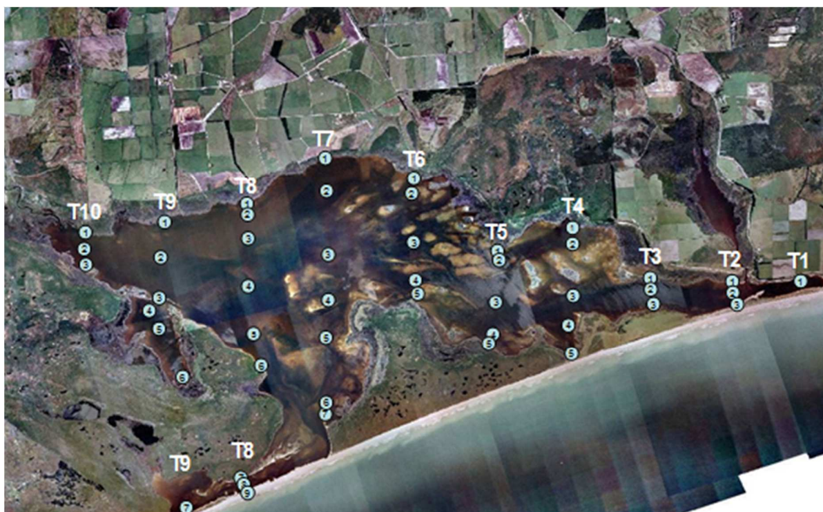
Figure 2-1: Geo-referenced survey sites located in Waituna Lagoon. Transects are numbered 1 to 10 from East to West and numbered on each transect in ascending order from North to South.
