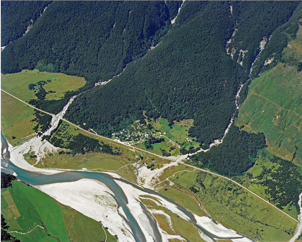
Figure 6.14 Oblique aerial view of debris-flow fans in the Makarora valley. Photograph by L Homer, 1996, GNS Science.
