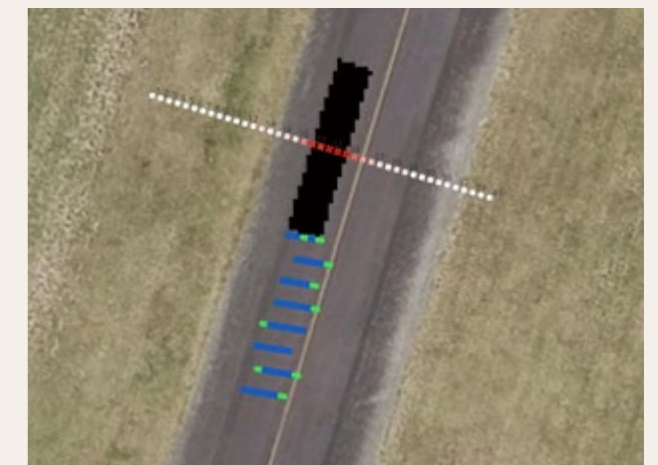
Spray deposition (red dots lots of spray/white dots no spray) relative to targets (ragged black boxes) on the Taupo taxiway. Blue dots are the spray nozzle actuation points (they're sampled at 10hz – hence gaps between line of blue dots). Most spray landed within .5m of the targets. Photos: James Griffith
