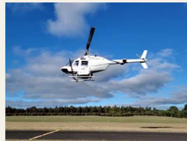
Helicopter autoboom for precision herbicide application Photo: James Griffith
