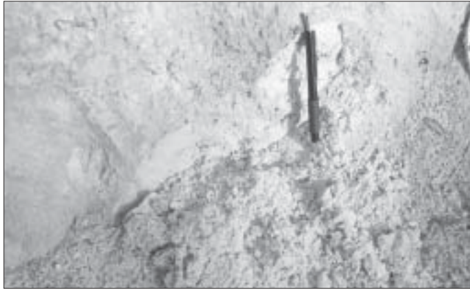
Figure 7. Exposure in cutting of medium-dense, fine-to-medium sand.
