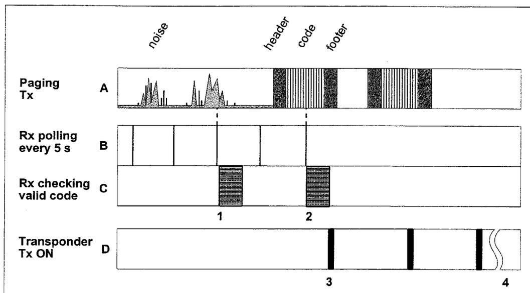
FIGURE 3. TRANSPONDER ACTIVATION TIMING. TRANSPONDER'S RECEIVER (Rx) POLLING EVERY 5 s (B) RESPONSE TO NOISE (C, 1) AND VALID PAGING TRANSMITTER (Tx) CODED SIGNAL (C, 2). TRANSPONDER'S TRANSMITTER ACTIVATED (D, 3) AND PULSES UNTIL TURNS OFF (D, 4) AFTER A SET DELAY.
