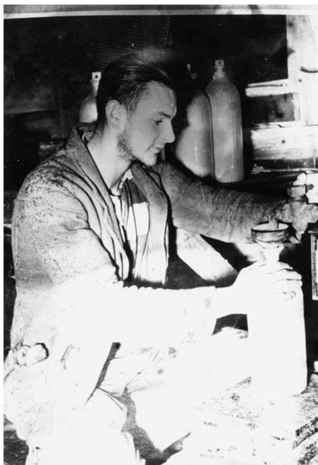
Figure 12: Dusty Miller filling a cast iron mercury flask; image held at the Whangarei Library
