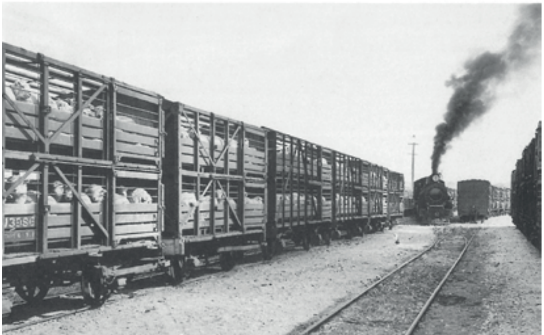
Figure 10. Omakau sheep, February 1960. All the planning of a chess move was required to position deckers for loading at Omakau during the height of the season. A locomotive was stationed there to assist with the requisite shunting and to take a daily train originating there. The J class wagons nearest the camera held 60 sheep, while the newer Jc class held 80. Photo: New Zealand Railways.
