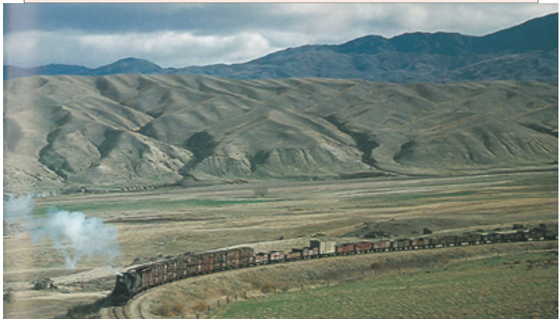
Figure 1. The struggle. The grade of Tiger Hill, rising 1 metre in every 50 travelled and extending for 5 kilometres, was a great struggle for trains on the Otago Central Railway. This train in 1964 would be well over the limit for one locomotive, except that half the wagons are returning empty. The month is May so the empty wagons have likely brought in coal in anticipation of winter. The 12 specialised wagons that are loaded – 10 with sheep and 2 with fruit – reflect the nature of the Central Otago local economy. Being so late in the season, these loadings are light. The key ingredients of this historic scene are the physical challenge of the long hill climb and the dramatic sheep-farmed landscape. Today, these same two values are still the key appeal for trail cyclists, who may also anticipate the hospitality that awaits them down the other side at Omakau. Photo: George Emerson.
