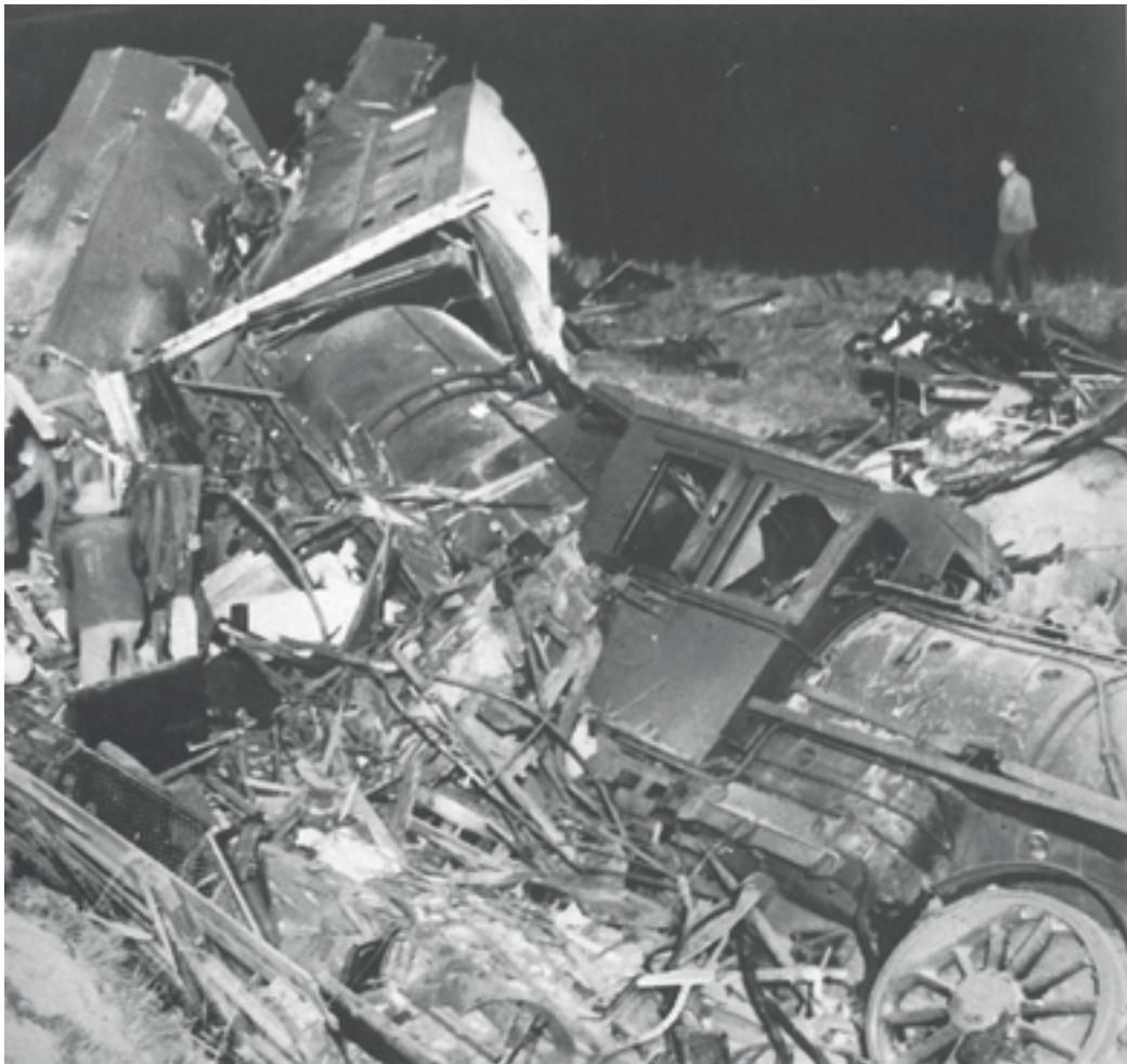
Figure A2.1. The carnage and high death toll of 23 was caused by the location within a cutting, which confined the carriages and caused them to crush up behind the locomotive. Photo: J.D. Mahoney collection.
